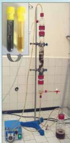
Textile wastewater treatment by Bjerkandera adusta in fixed-bed bioreactor. Ten cycles of degradation: colour, COD and toxicity were effectively reduced.
