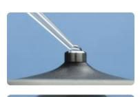
After the arm is closed, a sample column is formed.
